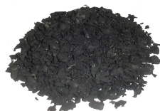
Rejected TDF with high steel content
