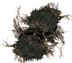
Rejected TDF with high steel content
